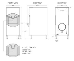
INSTALLATION NOTE: ALLOW 6" SPACE AT LEFT, BACK, AND RIGHT SIDES FOR VENTILATION AND UTILITY CONNECTIONS
