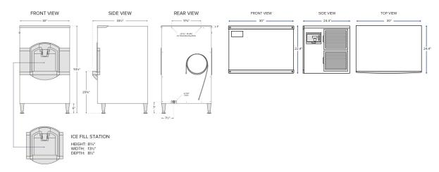
INSTALLATION NOTE: ALLOW 6" SPACE AT LEFT, BACK, AND RIGHT SIDES FOR VENTILATION AND UTILITY CONNECTIONS
