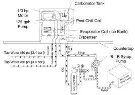
NOTE: This is a simplified schematic to show the basic operation of the beverage system.
