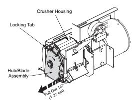
B. Pull the hub/blade assembly out of the housing approximately 1/2" (1.27 cm) to disengage the crusher axle from the motor shaft.
