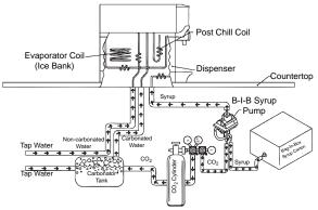
NOTE: This is a simplified schematic to show the basic operation of the beverage system.
