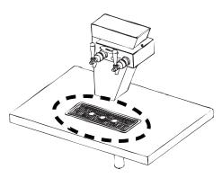
NOTE: The Blade Tower can be set up to use an existing drain or an optional drain can be ordered for use with the tower. The illustration above shows the optional flush mount drain setup (Part Number 020001388). If using the optional flush mount drain, be sure to plumb according to local codes.
