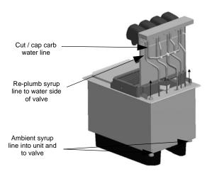
NOTE: Tapping into existing water line too close to the pump deck can result in starving the valve when the carbonator cycles. If a dedicated water line is not possible, tee into the existing water line as close to the source as possible.
