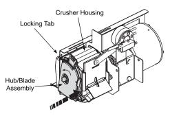
3. Once all blades are in the crusher housing you will need to align the crusher axle with the motor shaft. You can do this by turning the axle knob and pushing the blade assembly toward the motor until the hub/blade assembly is flush with the end of the crusher housing.
