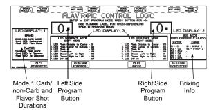
Mode 1 displayed above, allows you to select your carb/non-carb settings for dispense points N3 (Nozzle 3) through the left control board and/or N4 (Nozzle 4) with the right control board. Only nozzles N3 and N4 have the option to be a non-carb drink, N1 and N6 are carbonated only. Mode 1 is also used to set a 1 or 2 second dispense duration for flavor shots on N2 and N5 using their corresponding control board.
