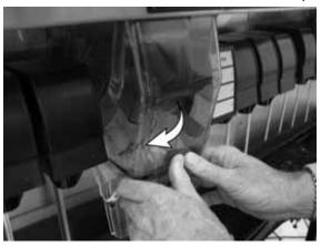
C. Rock top of the chute forward until top of chute clears unit.
