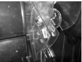
B. Grasp handle of the pin on the right side, pulling until the ice wheel is loose.
