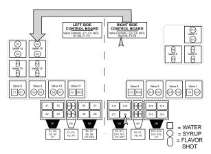
S9 (Syrup 9) on Valve 15 is the only syrup that does not correspond to the side it is mounted to. Both visually and functionally all other valves, touch pads, and dispense points correspond with the board on the same side to which they are attached.
