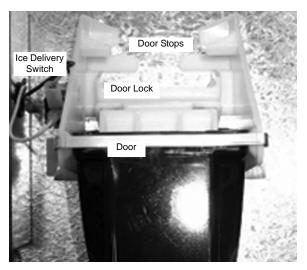
Begin by observing the chute by slowly pushing against the rocking chute. When the ice delivery switch clicks, measure the distance from the door stops on the rocking chute bracket to the door. The distance between the two must be no more than 1/4" (0.64 cm), but no less than 1/16" (0.16 cm).
