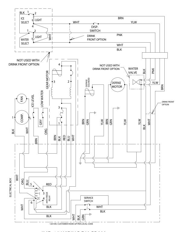
**IMD-15 WIRING DIAGRAM**
