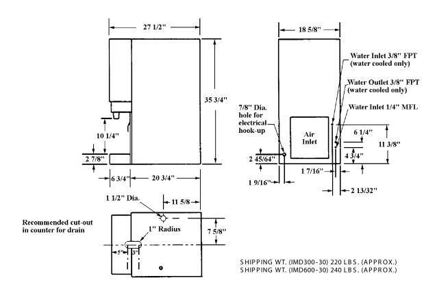
FIGURE 2. DIMENSION DRAWINGS (30 LBS.) IMD 300-30 AND IMD 600-30
