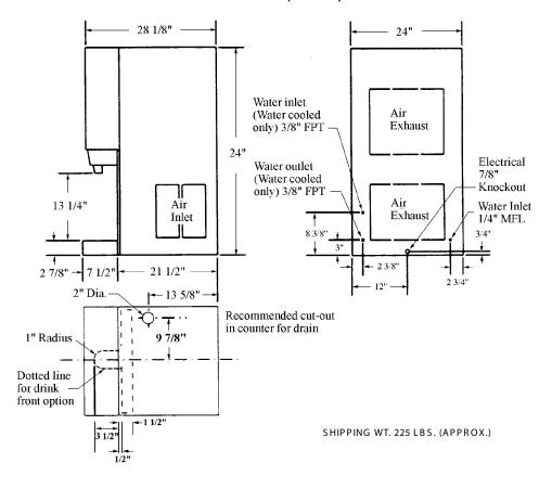
FIGURE 3. DIMENSION DRAWINGS (90 LBS.) IMD600-90
