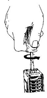
FIGURE 6. ADJUSTMENT SCREW
