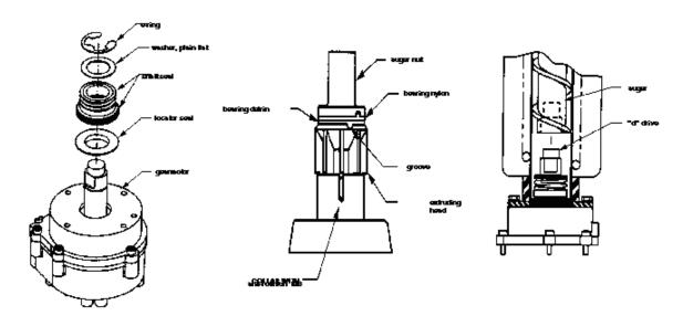
FIGURE 7. IMD 300 SHAFT SEAL
