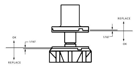
FIGURE 5. UPPER BEARING AND AUGER ASSEMBLY
